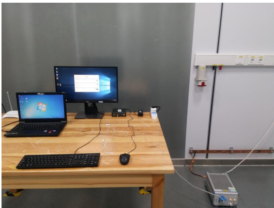
Fig. 4 Power line conducted emission setup photo
