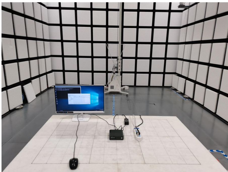
Fig. 2 Radiated emission setup photo(30MHz-1GHz)
