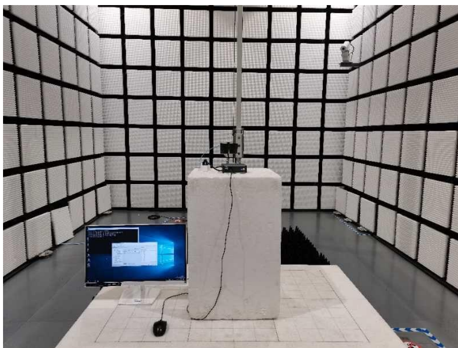
Fig. 3 Radiated emission setup photo(Above 1GHz)
