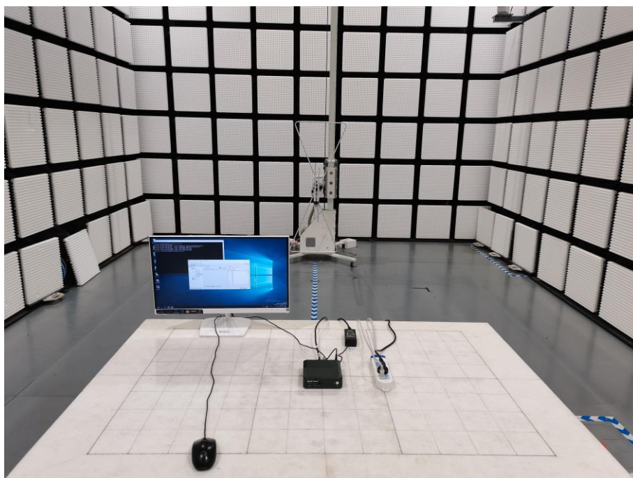
Fig. 2 Radiated emission setup photo(30MHz-1GHz)
