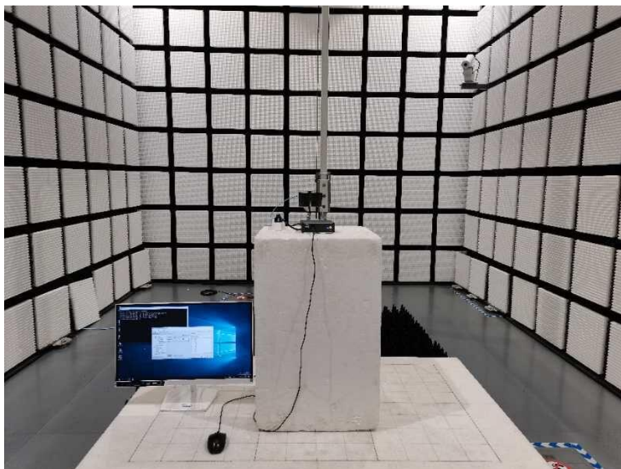
Fig. 3 Radiated emission setup photo(Above 1GHz)
