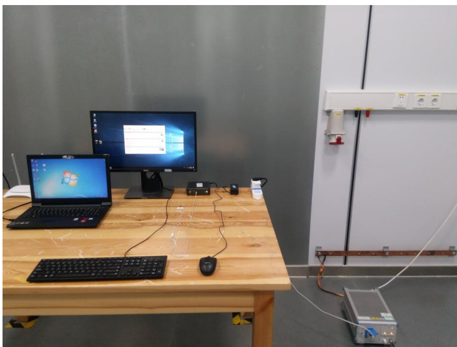
Fig. 4 Power line conducted emission setup photo
