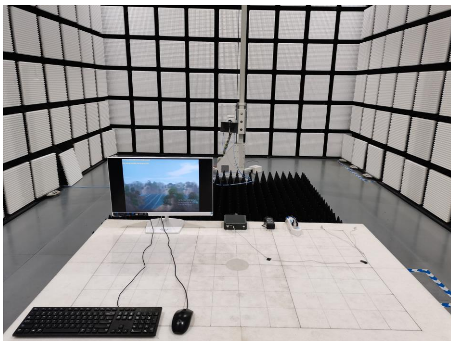
Fig. 2 Radiated emission setup photo(Above 1GHz)
