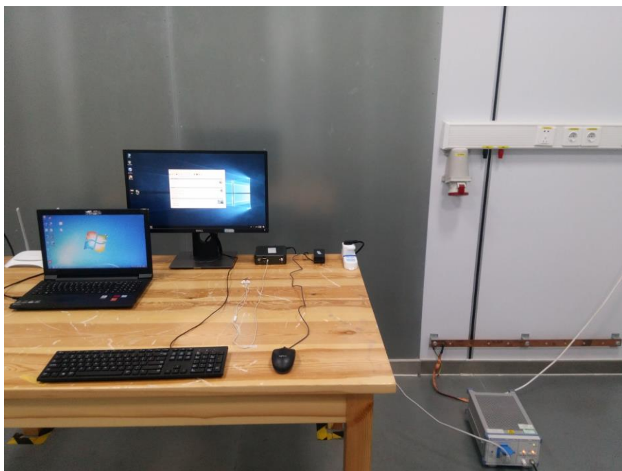
Fig. 3 Power line conducted emission setup photo
