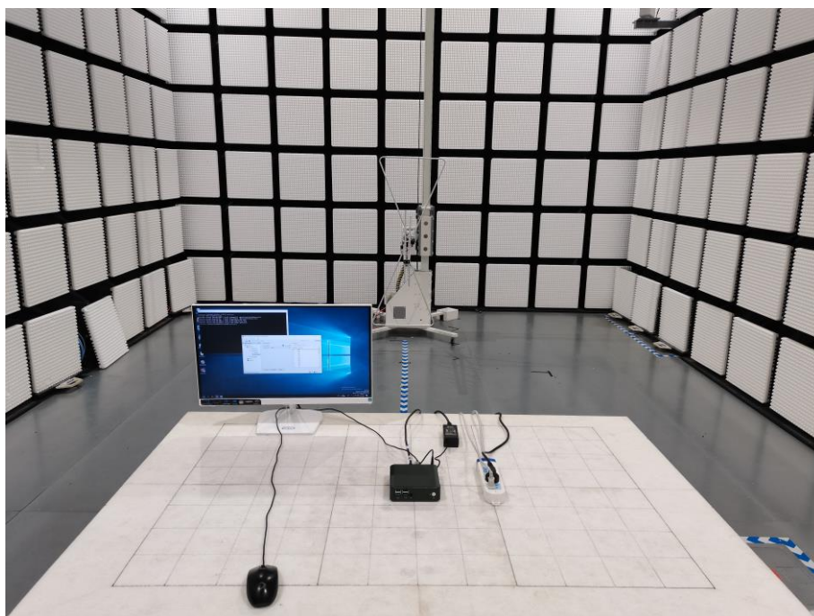
Fig. 1 Radiated emission setup photo(30MHz-1GHz)
